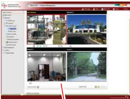
Video displays such as single camera, picture-in-picture, or quad can be easily built. Analog and IP cameras can be mixed on the same display. Telemetry and historical video browser controls are shown when these functions are available.
