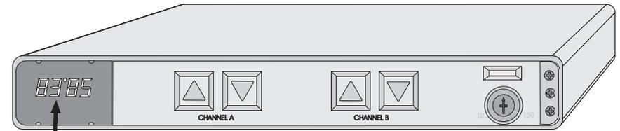
Display indicates the selected channel numbers. When no video signal is present, the display for that channel will not remain lit.
