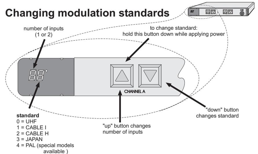
1. Using the supplied transformer, apply power while pushing the channel A "up" selector button. The unit will remain in the modulation standards programming mode until power is removed.
