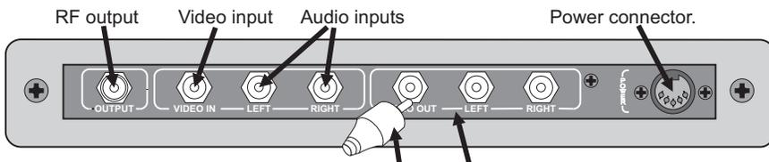
The model 6315 is a single channel MTS stereo video modulator. Stereo video sources (DVD players, LV players, VCRs) will provide stereo with dbx noise reduction on all TVs in the house. The 6315 is compatible with modern surround sound processors.
