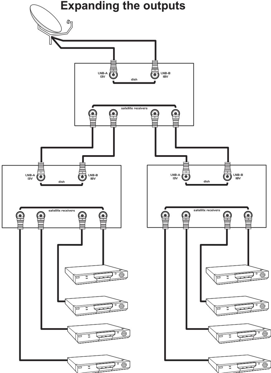
Adding a second multi-switch expands the system to six receivers. Adding a third multi-switch allows the use of up to eight satellite receivers. Do not cascade multi-switches more than 2 'layers' deep.
