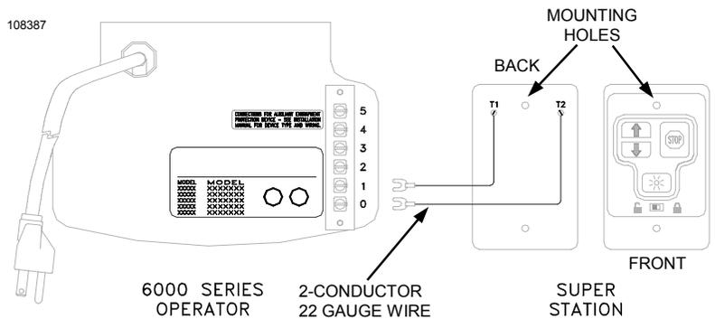
**WARNING: SOME LOCAL BUILDING CODES DO NOT ALLOW SURFACE WIRING. BE SAFE AND CHECK WITH YOUR LOCAL BUILDING INSPECTOR FIRST.**
