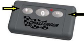
**4.** After the 10-digit code is entered, the LED will blink twice to confirm a valid code and remain off.
