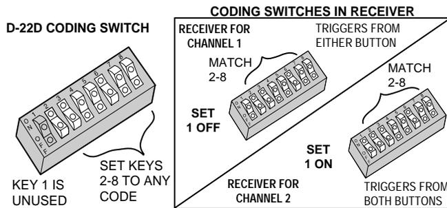
**STEP 2B Coding for two-channel receivers.** Pick any combination of OFF/ON codes and set them on switch keys 3-8 in the receiver. Match the same code on switch keys 3-8 in the transmitter. Set the transmitter switch 2 to OFF. Either button will activate Channel 1, both buttons will activate Channel 2. **2-Channel receiver switch keys 1 & 2 are unused and can be set in any position.**
