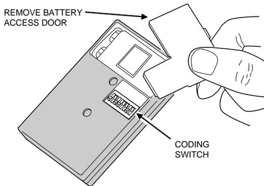
**STEP 2A Coding for single-channel receivers.** Pick any valid combination of OFF/ON codes and set them on switch keys 2-8 in the transmitter. Match the same code on switch keys 2-8 in the receiver. Set receiver switch key 1 to OFF for the receiver to activate from either transmitter button (Channel 1). Set receiver switch key 1 to ON for the receiver to activate only when both transmitter buttons are pressed (Channel 2).
