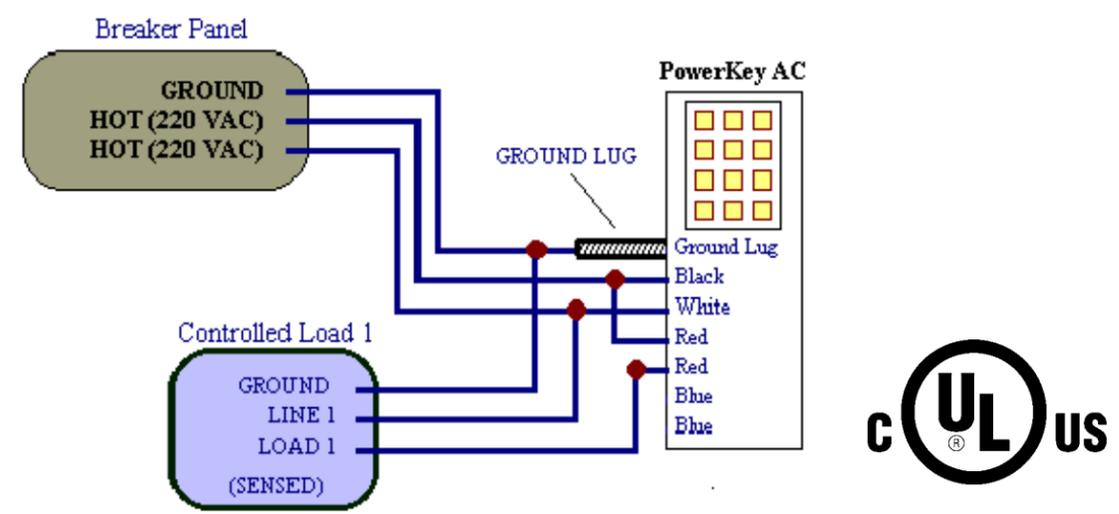
Wiring Diagram for PowerKey AC **without** an Auxiliary Device
