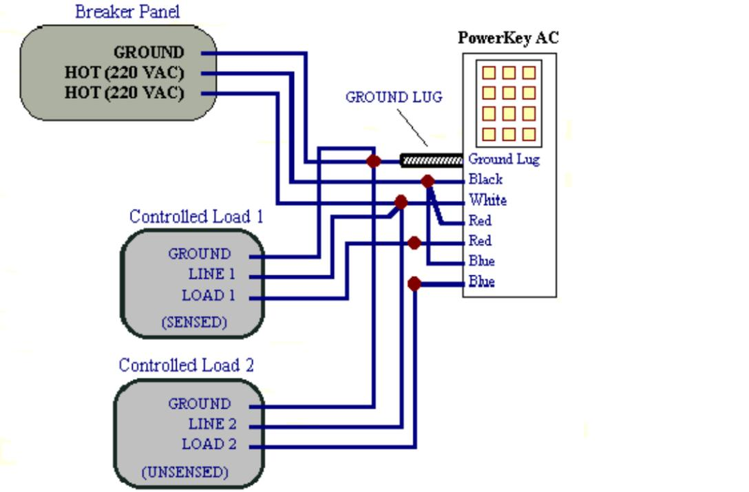
Wiring Diagram for PowerKey AC **with** an Auxiliary Device
