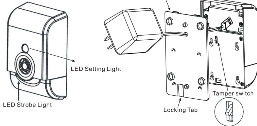
**NOTE:** This unit must be "included in the Network" **only where it will be permanently installed.** The proper operation of this node in the mesh network is dependent on it knowing its location with respect to other nodes. You cannot "test bench" configure this module, then install.
